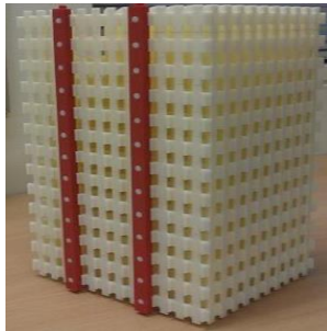
Figure 1. A prototype phantom measuring an effective volume of 200mm×200mm×300mm
